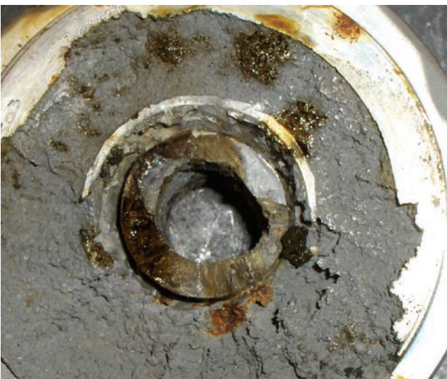
Typical cavitation damage
